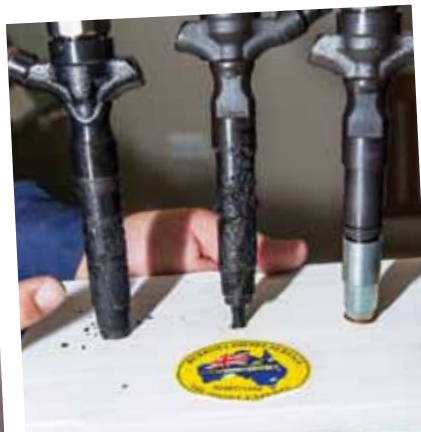
Notice the carbon build up on these D-4D injectors, it's a result of a failed injector seal, that separates combustion gases (carbon) from the engine oil
